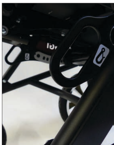
Attachment points, front according to ISO 7176-19
