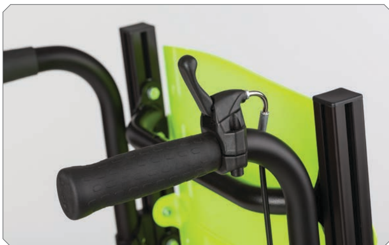
Release tilt in space mechanism.
