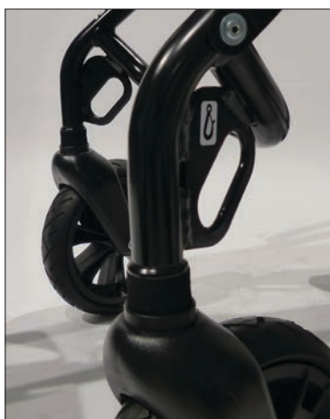
Attachment points, front according to ISO 7176-19
