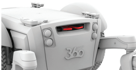
Figure 4.4a Magic 360 brake levers engaged
