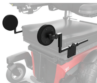
Figure 4.8a Kneepads on Centre Mounted Legrest
