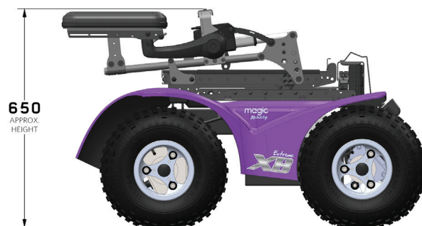
Figure 4.3d Extreme X8 Fold Forward height
