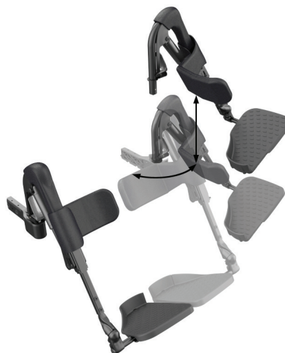
Figure 4.2c Swingaway Legrest showing removal action
