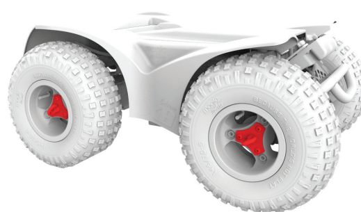
Figure 5.2d Extreme X8 lifting points (sold separately)
