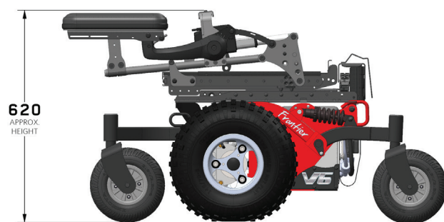
Figure 4.3c Frontier V6 and V4 Fold Forward height
